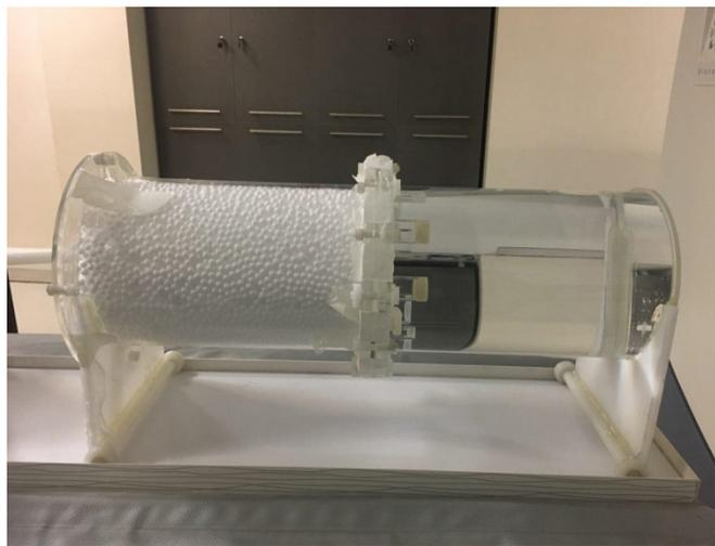
**Figure 2.** The phantom which was built to study the respiratory motion. As it is seen the phantom is connected to a system which mimics the respiratory pattern as an oscillatory motion. The amplitude of the motion is 4.5 cm in 4.5 seconds as it is in real respiration.
