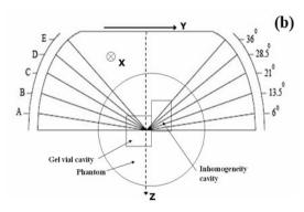
Figure 1. Phantom placed in a Gamma Knife unit (model 4C) for irradiation (a) and the schematic view of the irradiation experimental set-up for the 8 and 18 mm collimator helmet (b).
