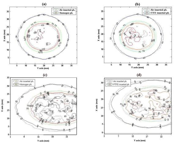
**Figure 5.** 2D dose distribution in axial plane in irradiation with 18 mm collimator of GK unit obtained using simulation (a and b) and PAGAT Polymer gel dosimeter (c and d). Dashed lines are isodose lines in air inserted phantoms and full lines are isodose lines in homogeneous (a and c) or PTFE inserted phantoms (b and d).
