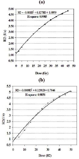
Figure 2. R2-dose curve of PAGAT polymer gel dosimeter for 8 mm (a) and 18 mm collimators of GK unit (b).
