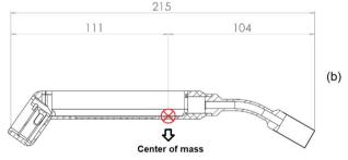
Fig. 2 a The GammaPen body design and  ${\bf b}$  the position of the center of mass
