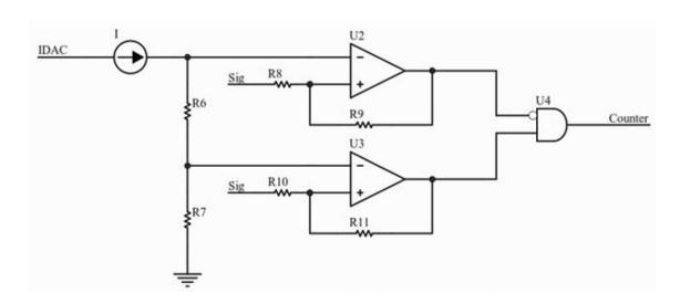
Fig. 5 Simplified circuit schematic of analog peak detection
