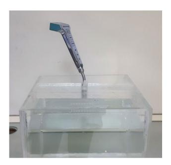
Fig. 6 Experimental measurements setup for NEMA NU3 evaluation in a scattering medium using a water bath with dimensions of 25 cm  $\log \times 25$  cm wide  $\times 20$  cm deep
