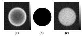
**Figure 3.** Illustration of reconstruction artifact resulting from lack of attenuation correction for uniform distribution of activity in a cylindrical phantom. (a) Reconstructed image without attenuation correction. (b) Uniform attenuation map at 511 keV. (c) Same slice as (a) after applying attenuation correction. Reprinted with permission from ref. [20].
