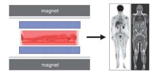
**Figure 18.** Concept of whole-body PET/MRI scanner, and images that such a system might produce (PET image courtesy of Siemens Medical Solutions; whole-body T1-weighted MR image courtesy of Dr. Heinz-Peter Schlemmer, University of Tubingen).Reprint with permission from ref. [118].
