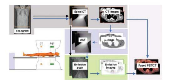
**Figure 4.** Principle of CT-based attenuation correction method on commercial PET/CT scanners. Reprinted with permission from ref. [34].
