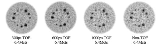
**Figure 17.** Reconstructed images for the central slice in the 27-cm phantom. These images are for a fixed count statistics (6.4 Mcts). Moving left to right the images are: 300 ps TOF scanner, 600-ps TOF scanner, 1000-ps TOF scanner, and non-TOF scanner. Same scan times lead to improved image quality in a TOF scanner with better timing resolution. Reprint with permission from ref. [123].
