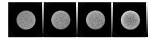
**Figure 9.** Reconstructed images of Monte Carlo simulated emission data corrected for attenuation using from left to right: CAC, CTAC primary, CTAC total fan-beam and CTAC total cone-beam. Reprint with permission from ref. [43].
