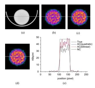
Fig. 7. Transaxial images of the uniform cylindrical phantom showing (a) CT image (b) Uncorrected PET image (c) CT-based attenuation corrected PET image using the bilinear energy-mapping method (d) Attenuation corrected PET image using the quadratic energy-mapping method, and (e) Corresponding horizontal profiles through images shown in (b)–(d).
