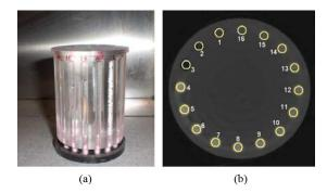
Fig. 1. (a) Photograph of the specially designed polyethylene cylindrical phantom containing 16 cylindrical holes (b) Transverse CT image of the calibration phantom showing the location of defined VOIs.
