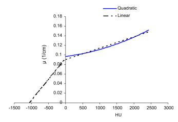
Fig. 2. Representative plots of bilinear and quadratic fitting of the calibration curves at 70 kVp and 275  $\mu$ A.
